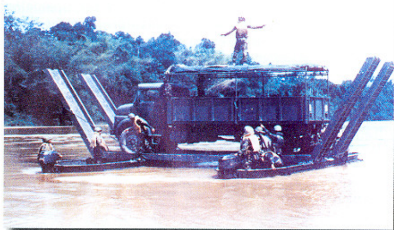
Light Raft (Catamaran) in support of River Crossing operation
