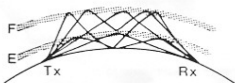
Typical multimoded propagation at frequency f_1
